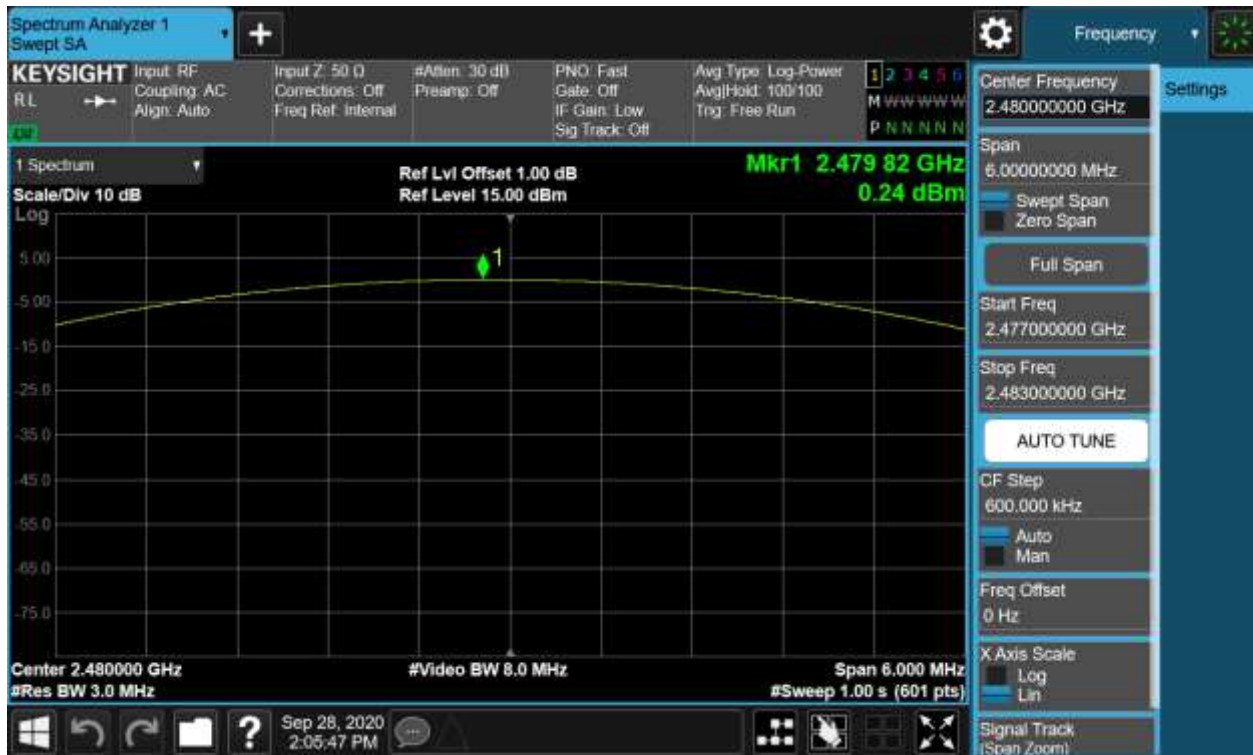
Figure 9: Maximum Conducted Output Power, 2480MHz, 8-DPSK
