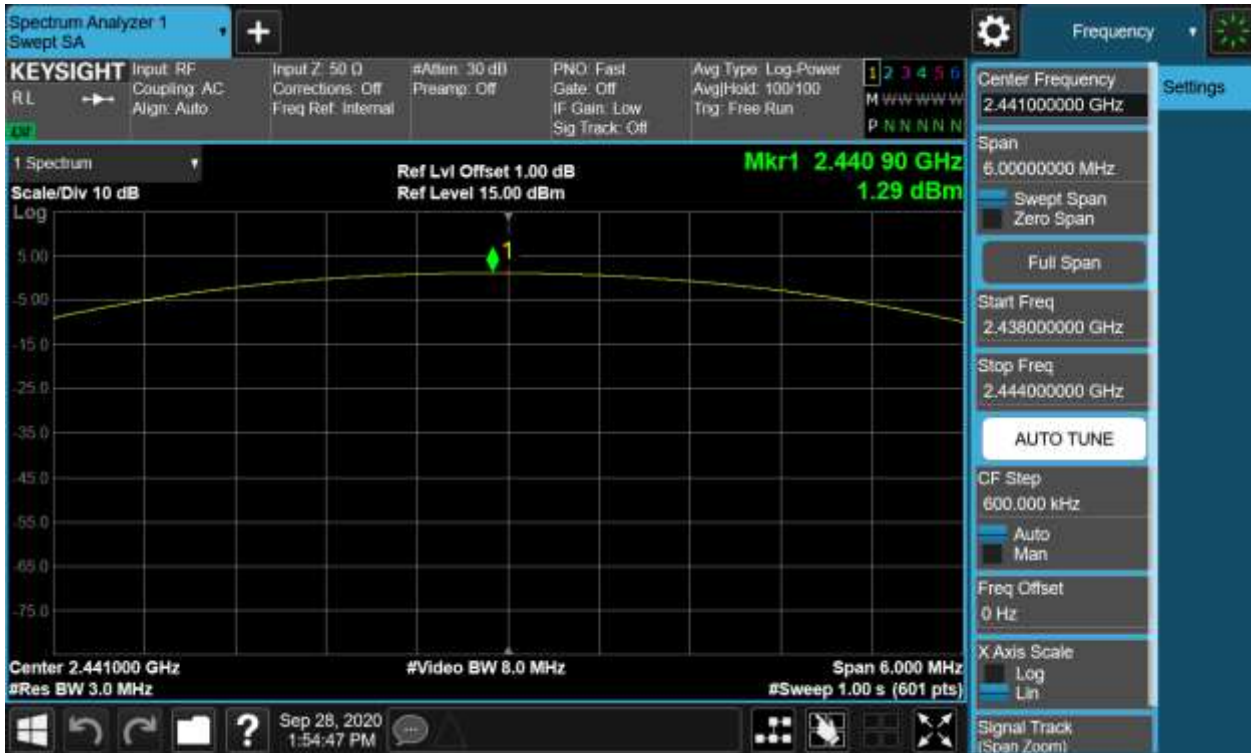
Figure 5: Maximum Conducted Output Power, 2441MHz, \pi/4 -DQPSK
