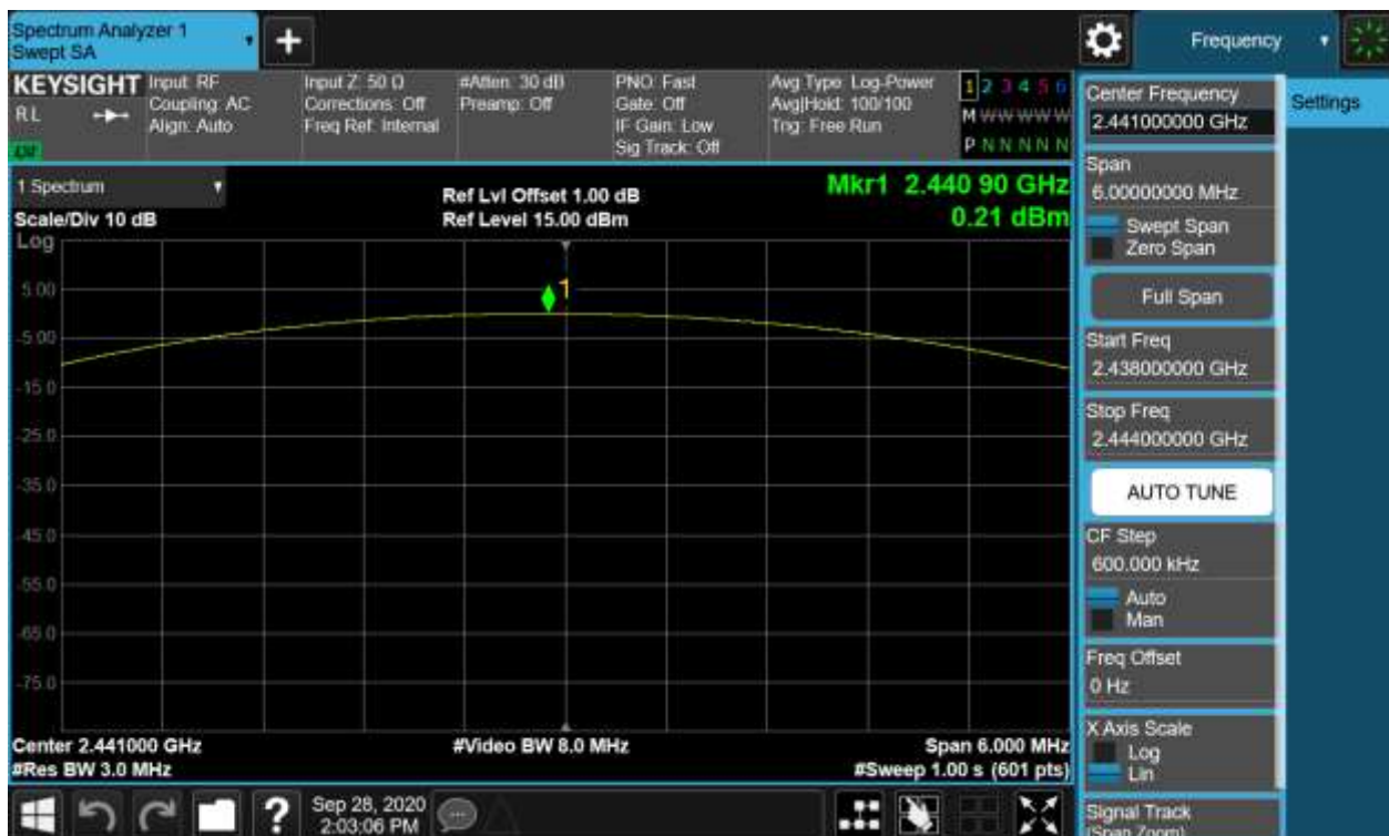
Figure 8: Maximum Conducted Output Power, 2441MHz, 8-DPSK
