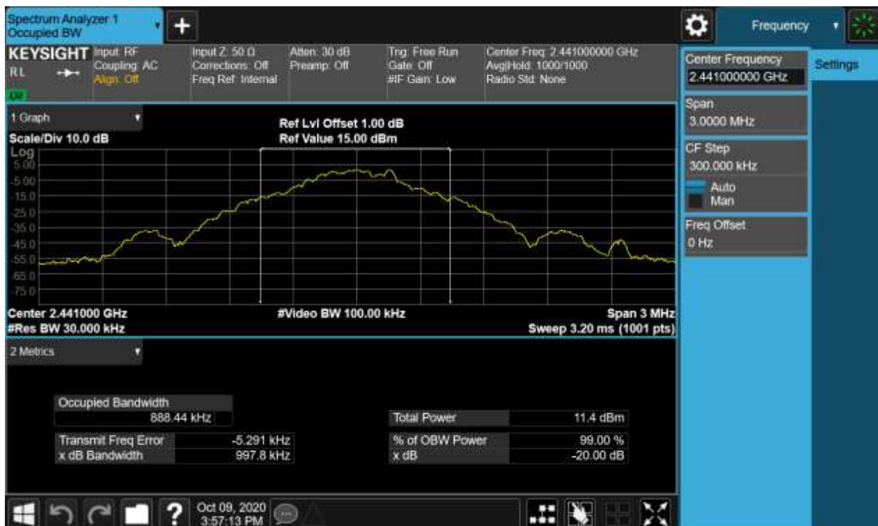
Figure 11: 20dB Bandwidth and 99% Bandwidth, 2441MHz, GFSK
