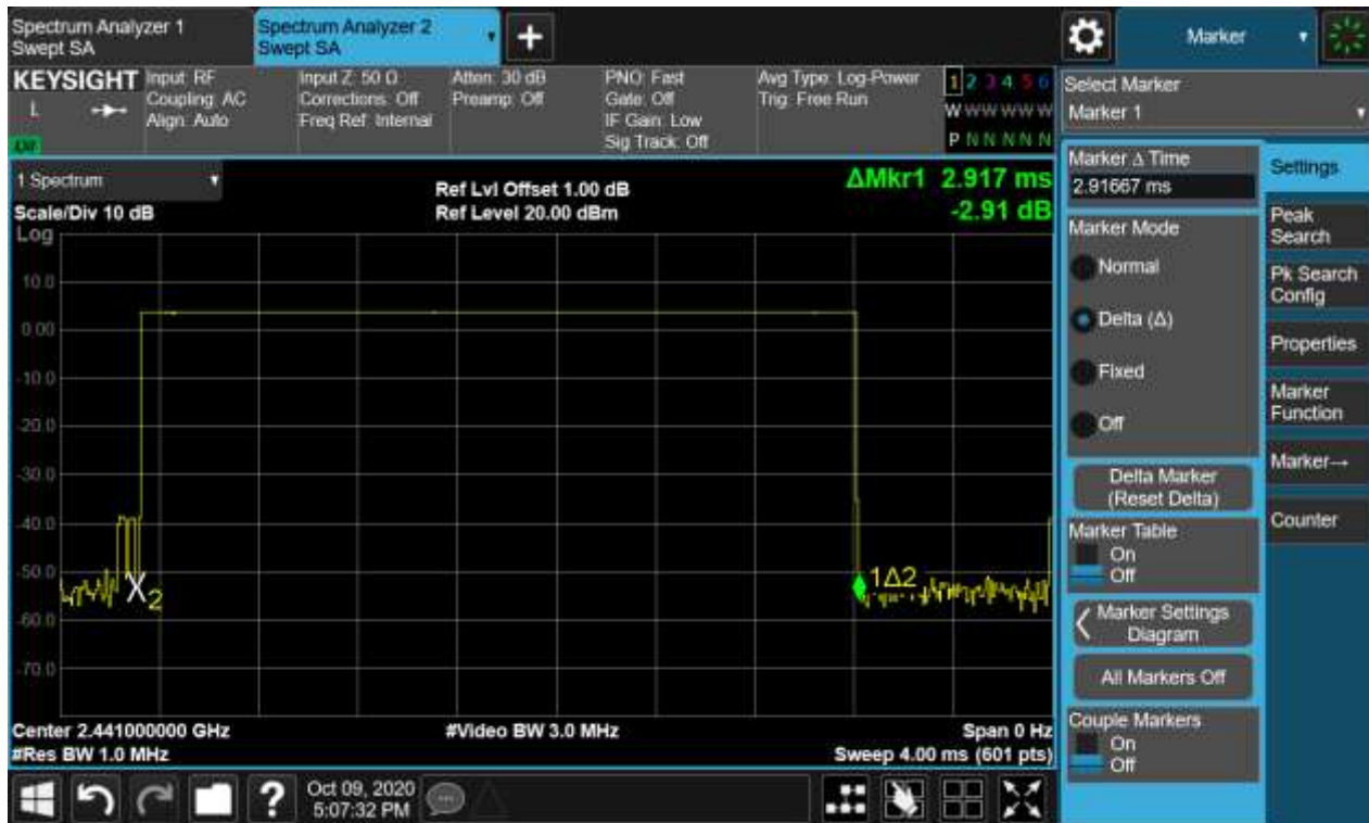
Figure 30: Time of Occupancy, 2441MHz, GFSK DH5
