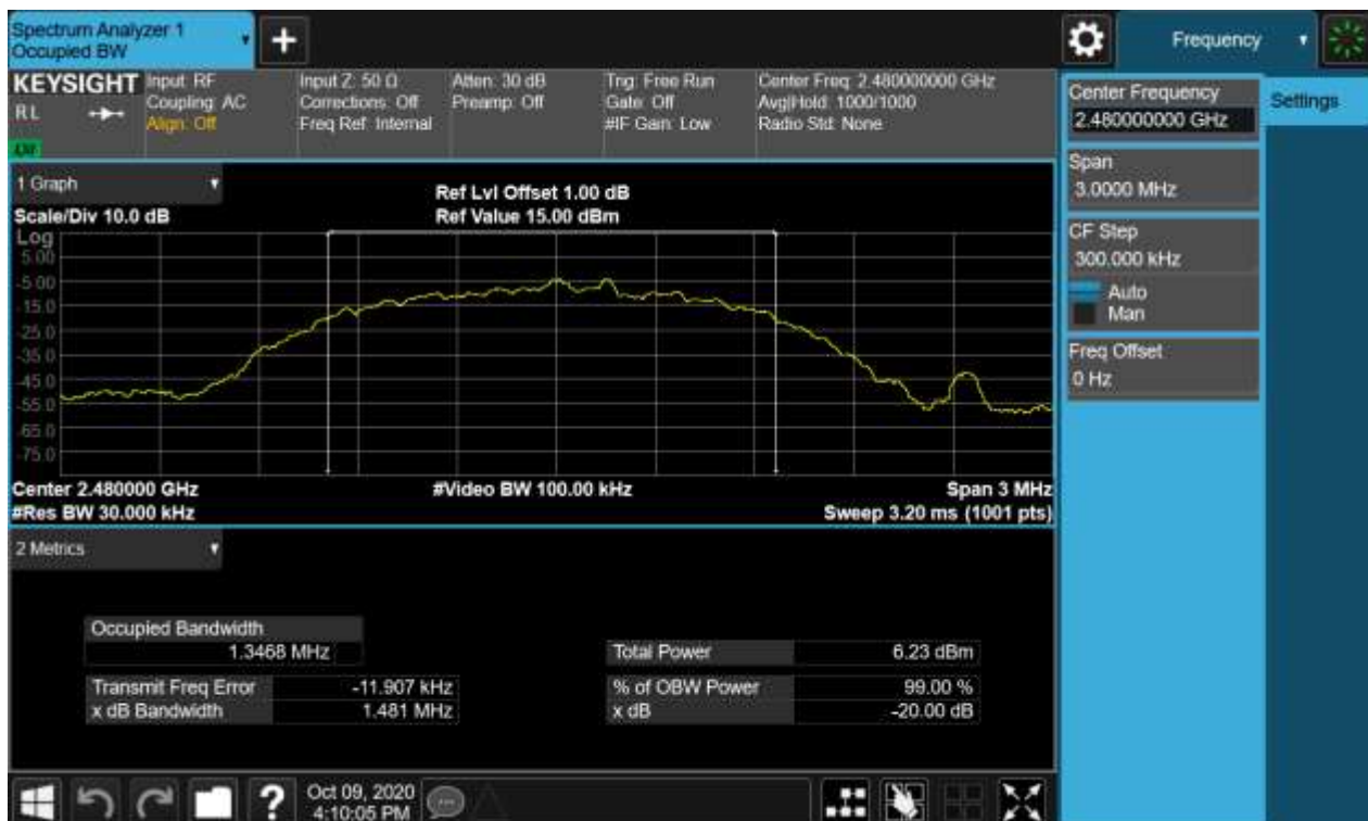
Figure 15: 20dB Bandwidth and 99% Bandwidth, 2480MHz, 8-DPSK
