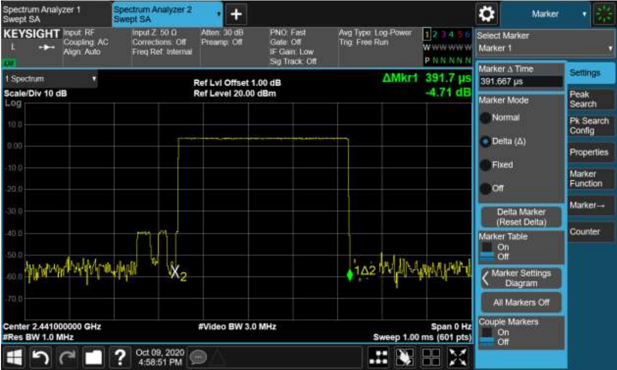
Figure 28: Time of Occupancy, 2441MHz, GFSK DH1
