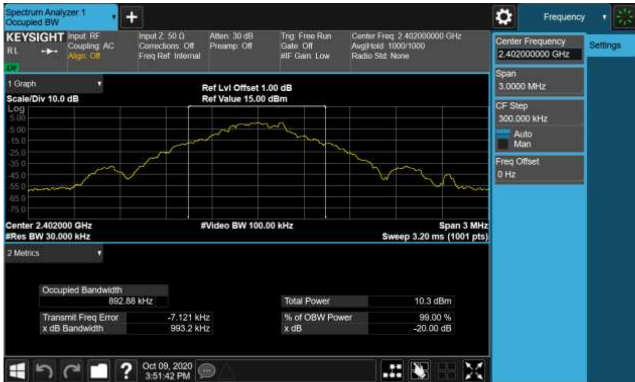
Figure 10: 20dB Bandwidth and 99% Bandwidth, 2402MHz, GFSK
