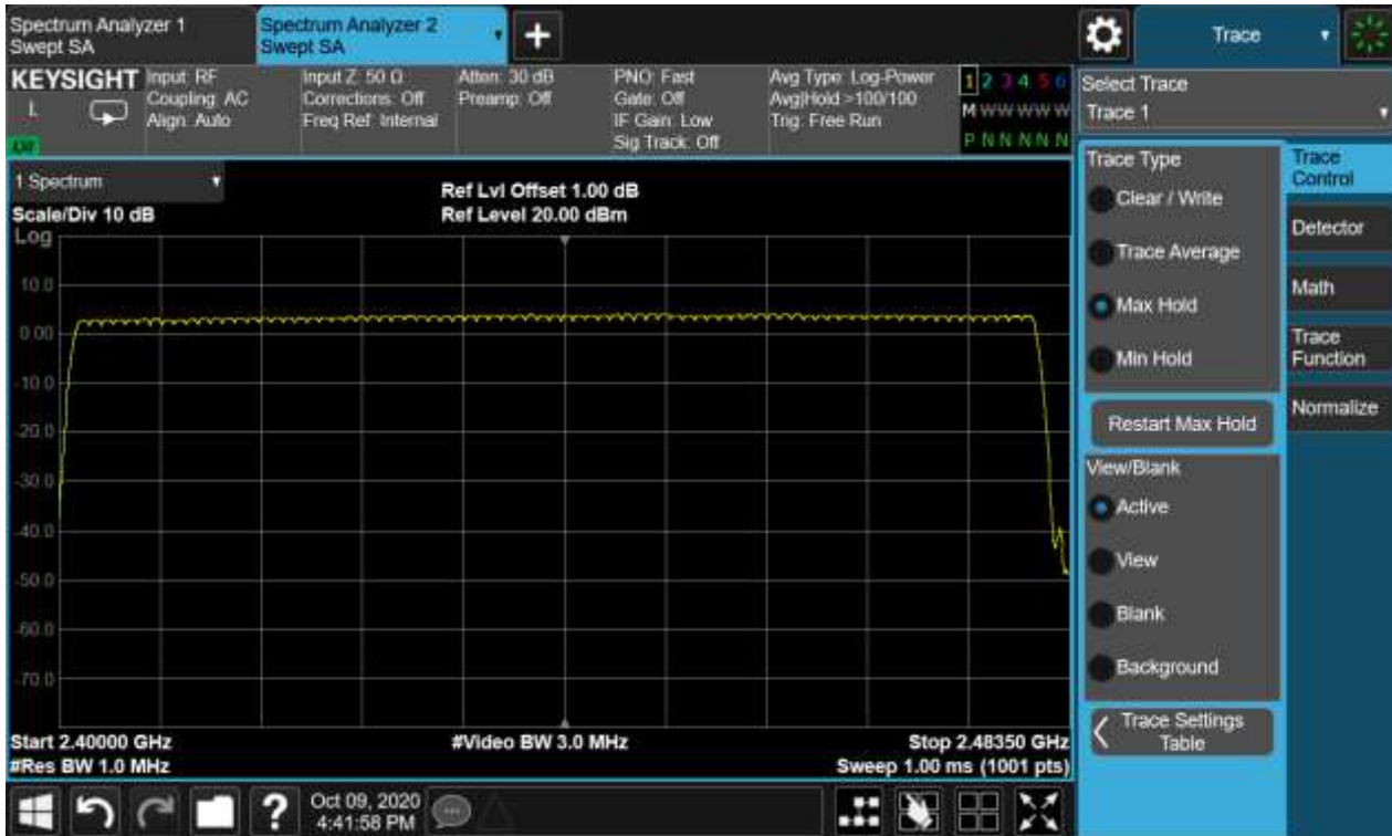
Figure 27: Number of Hopping Frequency, Hopping Mode, 8-DPSK
