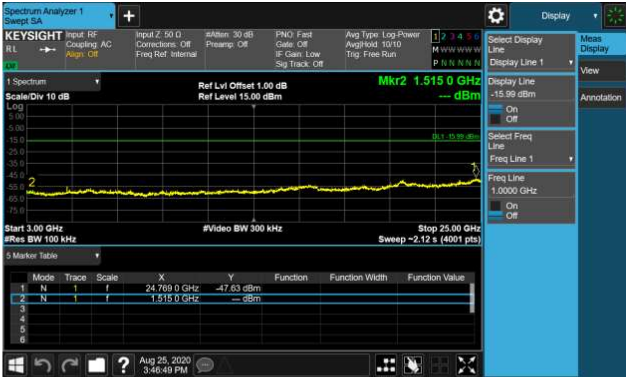
Figure 19: Conducted Spurious Emission & Authorized-band band-edge, 2402MHz, 8-DPSK Carrier Level
