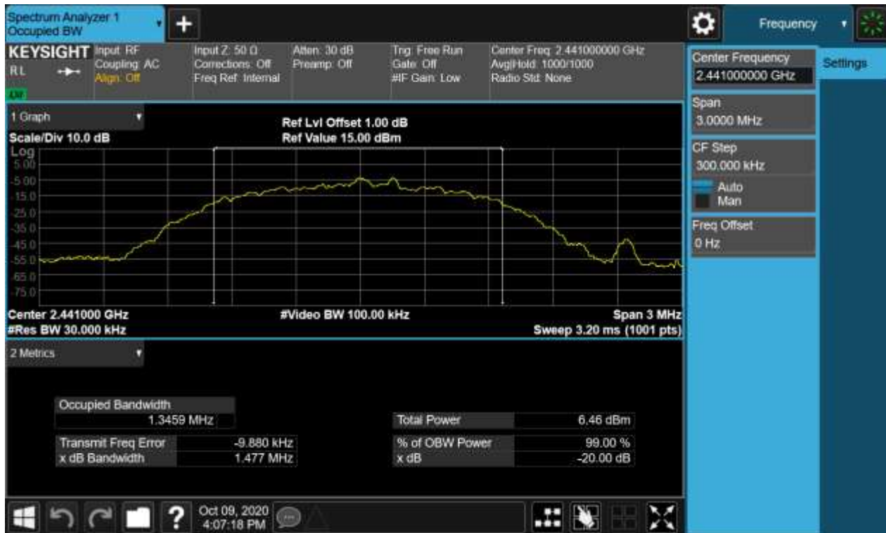
Figure 14: 20dB Bandwidth and 99% Bandwidth, 2441MHz, 8-DPSK
