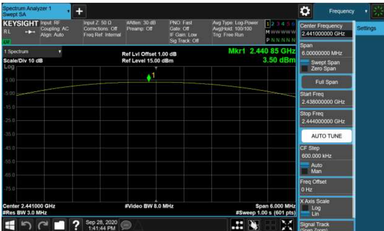
Figure 2: Maximum Conducted Output Power, 2441MHz, GFSK
