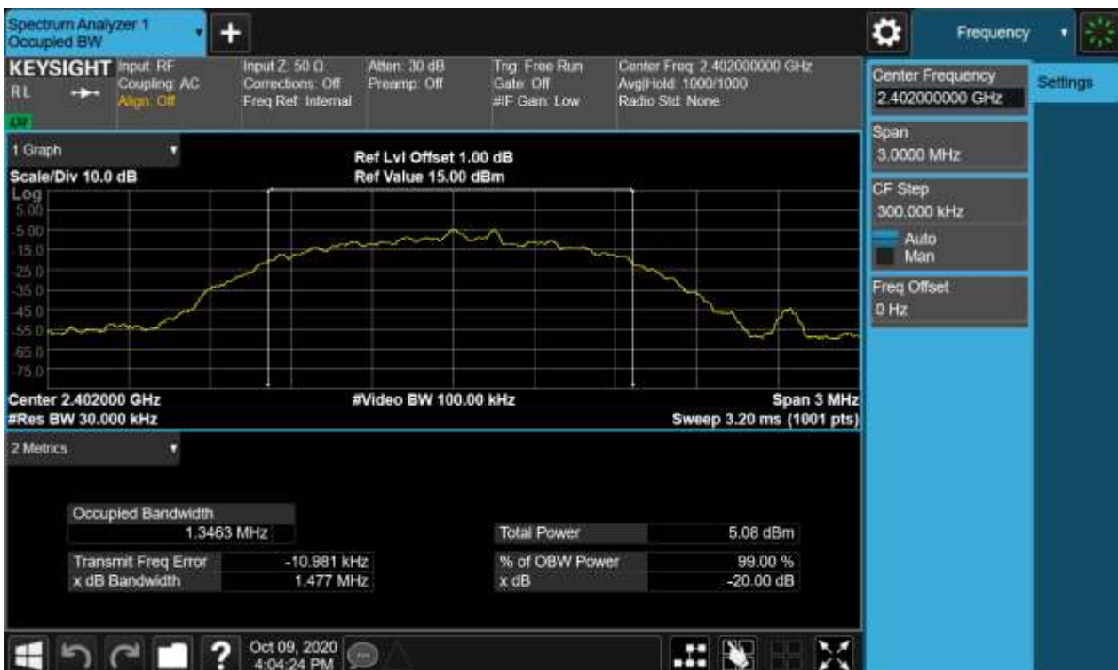
Figure 13: 20dB Bandwidth and 99% Bandwidth, 2402MHz, 8-DPSK
