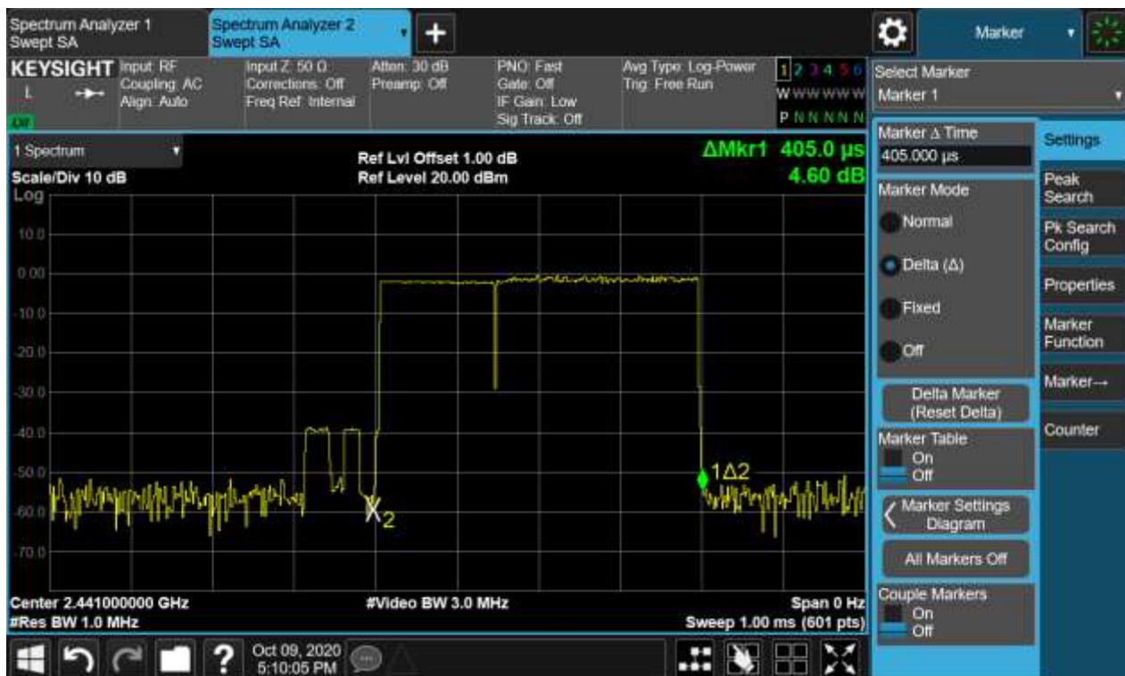
Figure 31: Time of Occupancy, 2441MHz, 8-DPSK DH1
