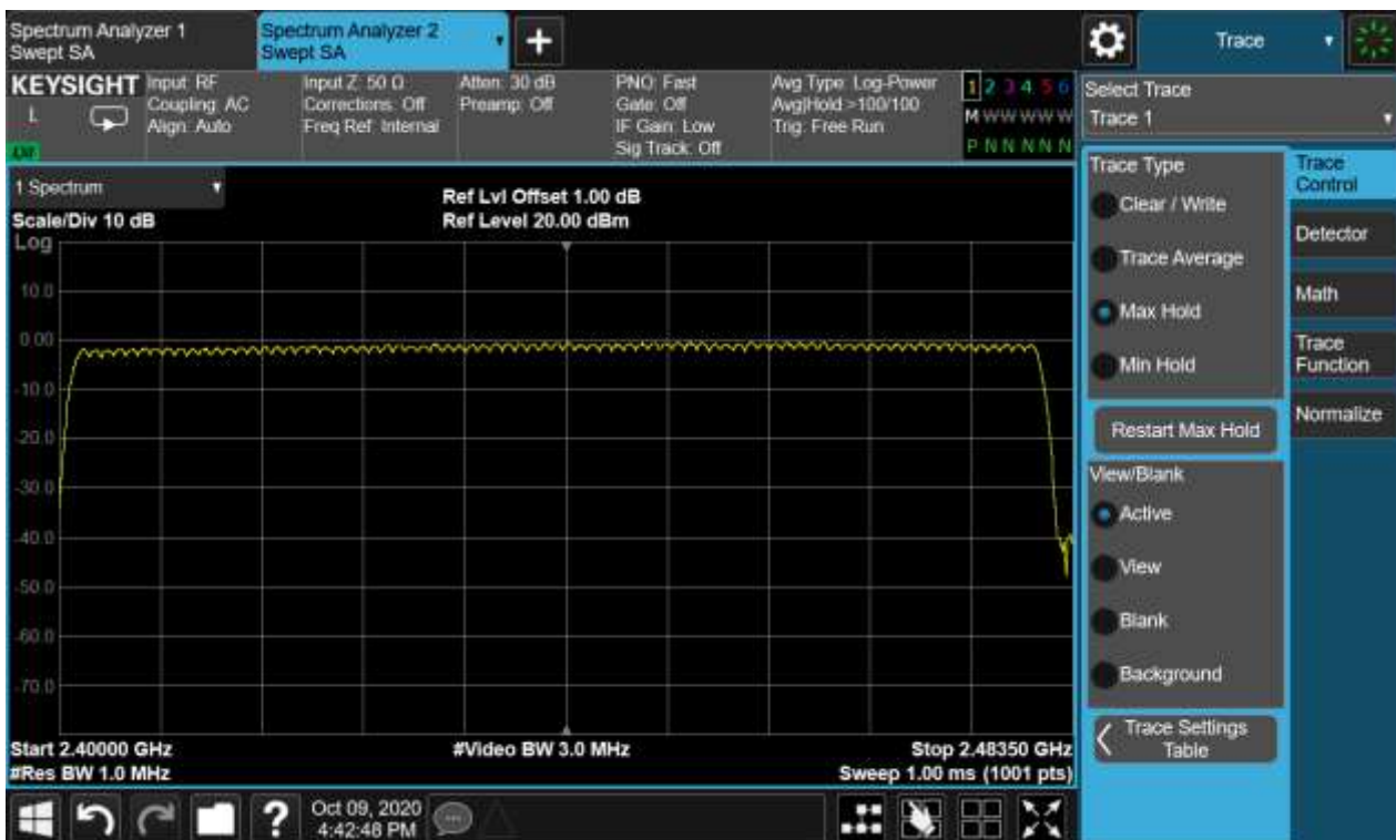
Figure 27: Number of Hopping Frequency, Hopping Mode, 8-DPSK
