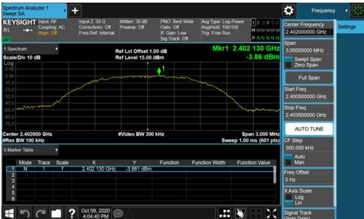
Figure 19: Conducted Spurious Emission & Authorized-band band-edge, 2402MHz, 8-DPSK Carrier Level
