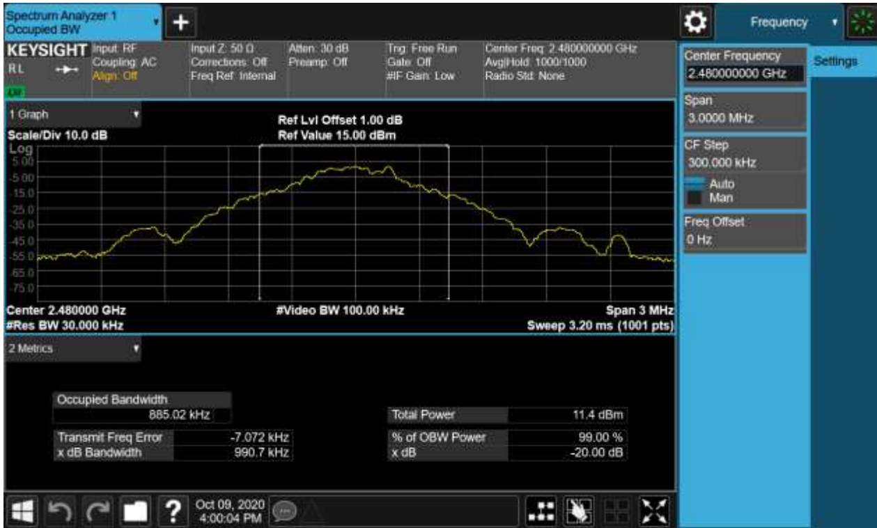
Figure 12: 20dB Bandwidth and 99% Bandwidth, 2480MHz, GFSK
