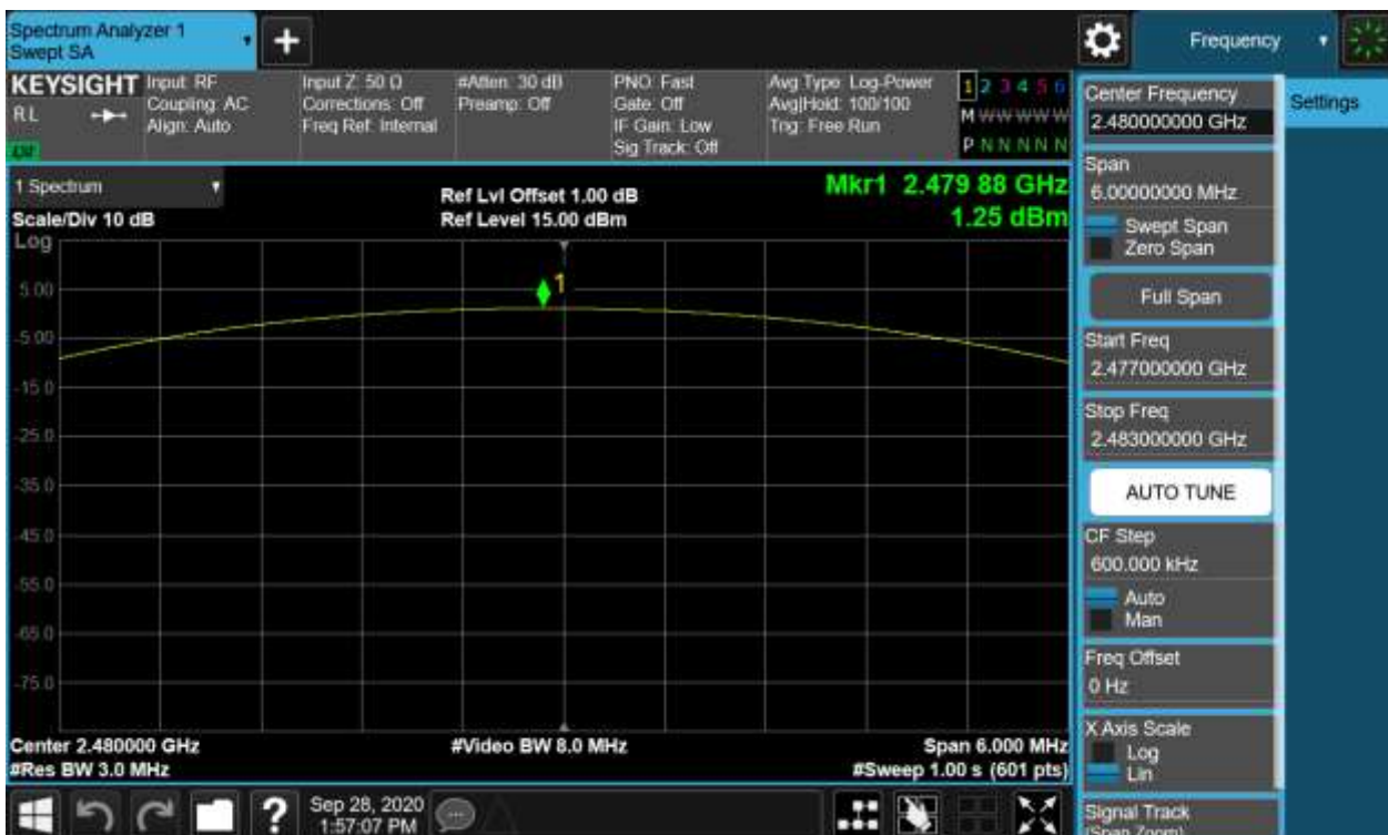
Figure 6: Maximum Conducted Output Power, 2480MHz, \pi/4 -DQPSK
