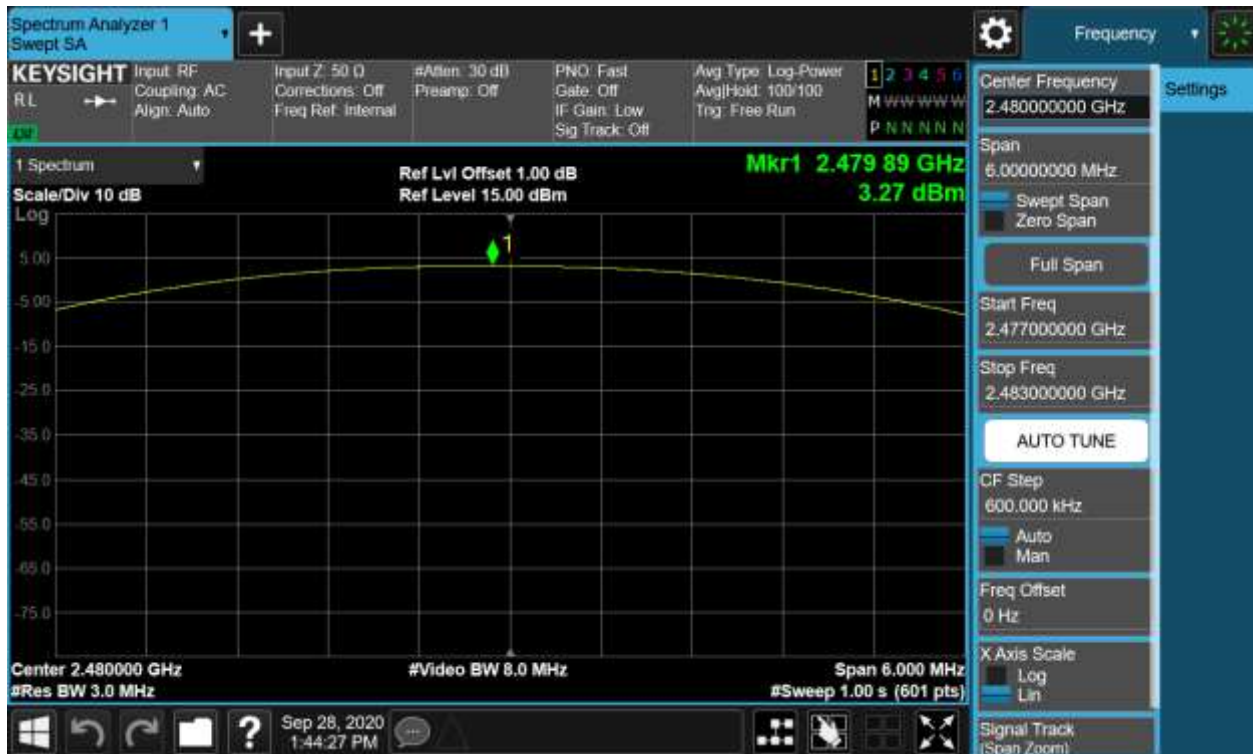
Figure 3: Maximum Conducted Output Power, 2480MHz, GFSK
