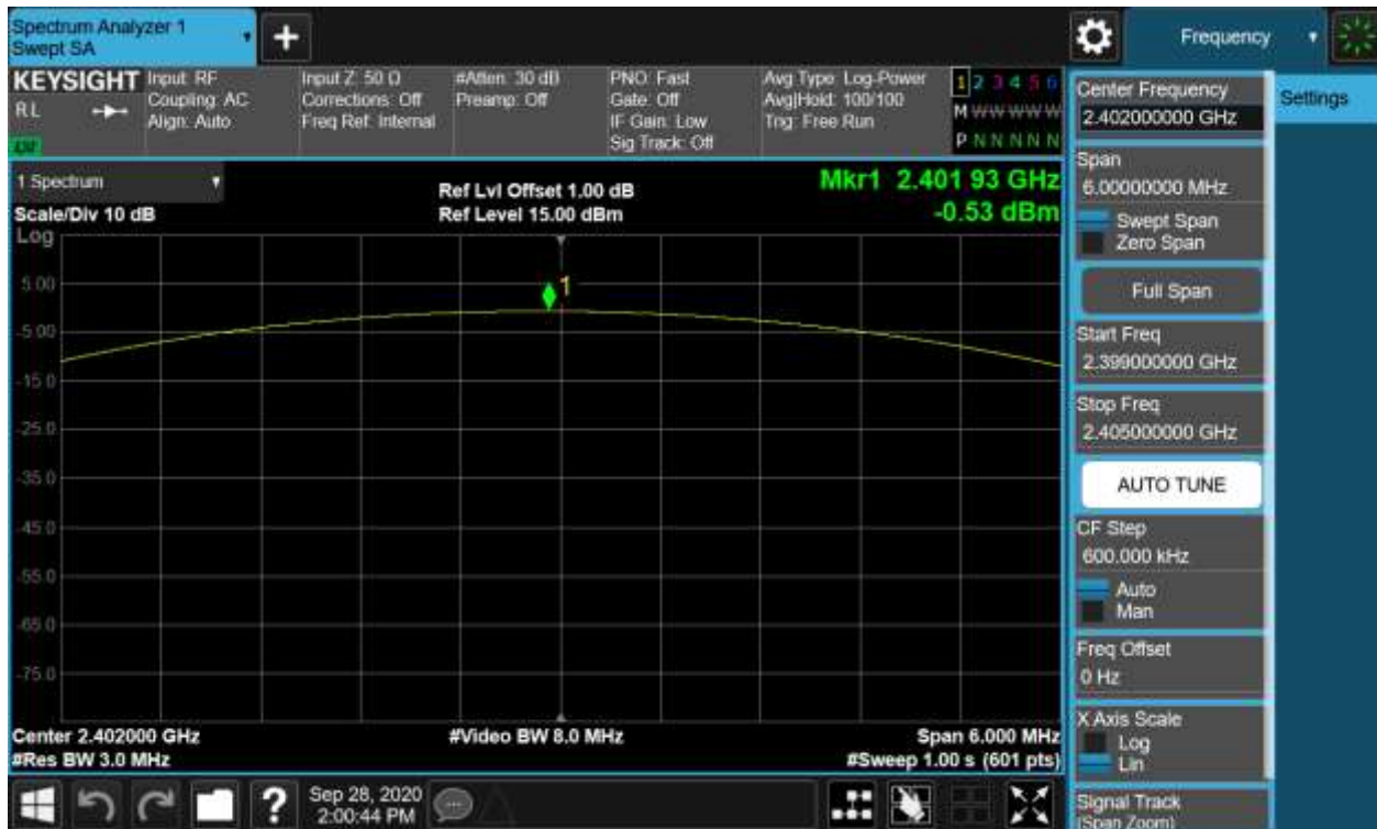
Figure 7: Maximum Conducted Output Power, 2402MHz, 8-DPSK
