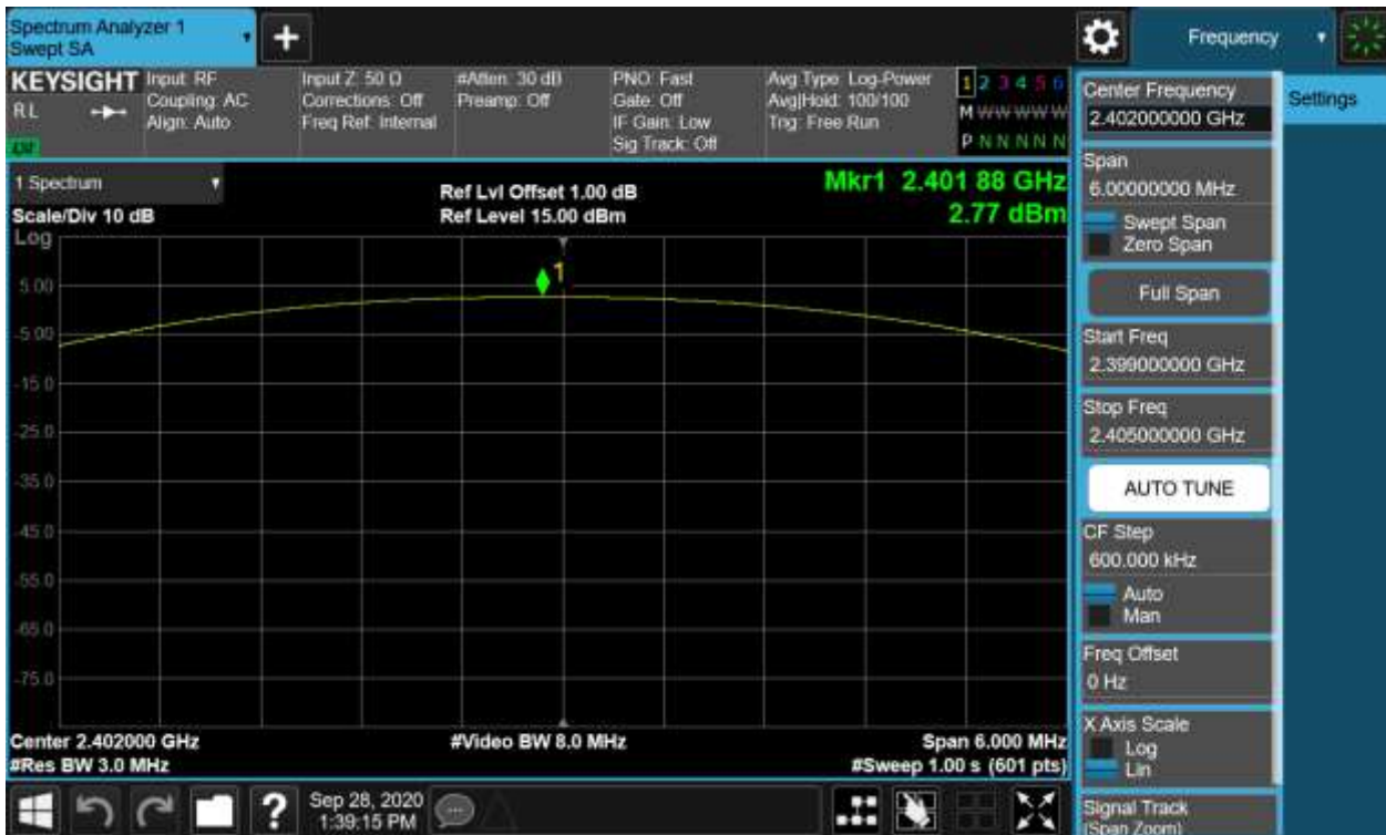
Figure 1: Maximum Conducted Output Power, 2402MHz, GFSK
