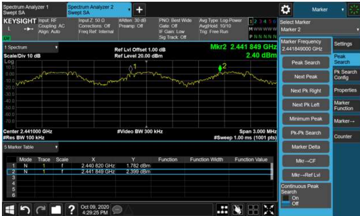
Figure 25: Hopping Frequency Separation, Hopping Mode, 8DPSK
