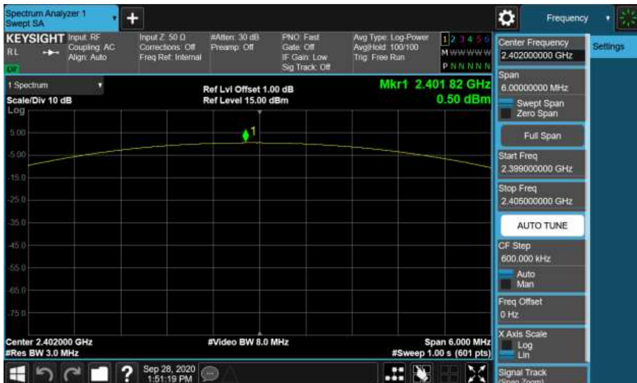
Figure 4: Maximum Conducted Output Power, 2402MHz, \pi/4 -DQPSK
