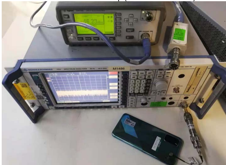
RF Conducted Test setup (BT/WIFI)
