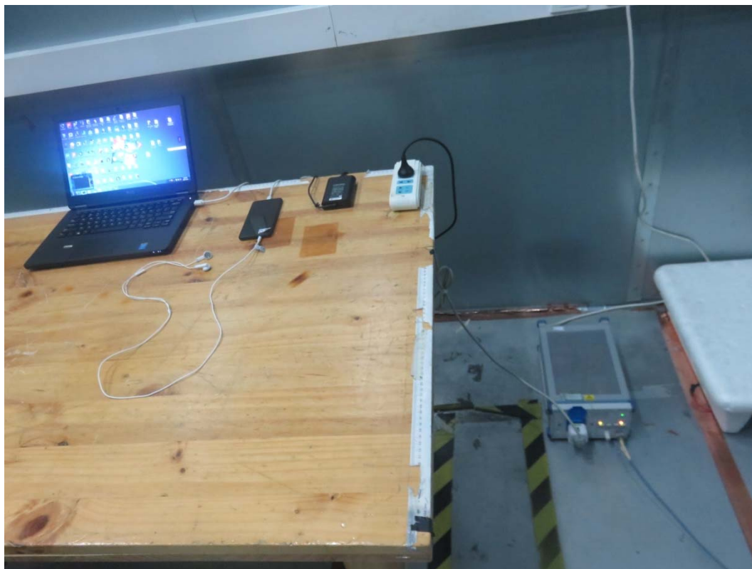
Picture 2 Conducted Emission Test Setup
