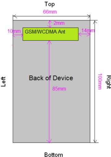
Note: Manufacture have declared that the safe distance is 15mm at the operation manual, so we did SAR test at 15mm.
