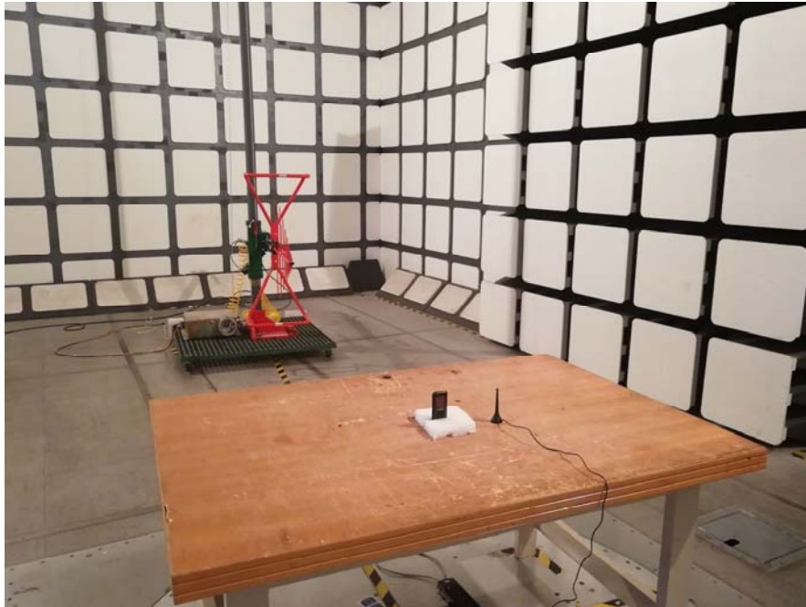
Radiated Emissions View (Below 1 GHz)
