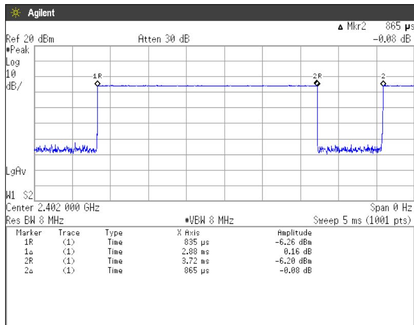
$$\text{Duty Cycle} = \text{Ton} / (\text{Ton} + \text{Toff}) = 2880[\mu\text{s}] / (2880[\mu\text{s}] + 865[\mu\text{s}]) = 76.90[\%]$$
