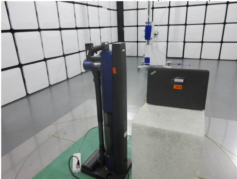
RADIATED RF MEASUREMENT SETUP (30MHz ~ 1 GHz)
