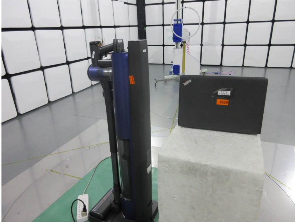
RADIATED RF MEASUREMENT SETUP (30MHz ~ 1 GHz)
