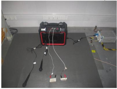
1.2 Radiated Spurious Emissions Test Setup
