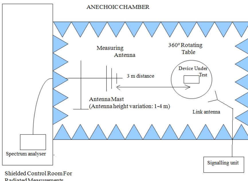
Radiated measurements above 1 GHz.
