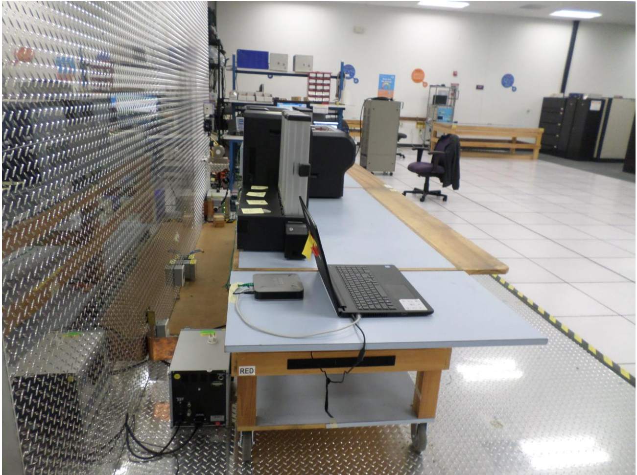
Figure 4: Conducted Emissions, Voltage - Setup Rear View
