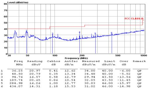
Note: 1. All readings are Quasi-peak values. 2. Measured= Reading + Antenna Factor + Cable Loss
