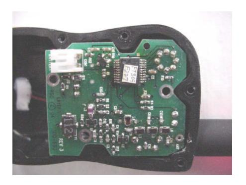
Photo 5. PCB Board Solder Side
