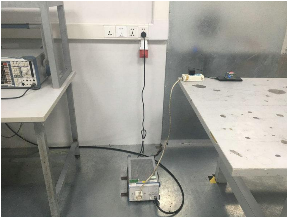
Photo of Conducted Emission Measurement
