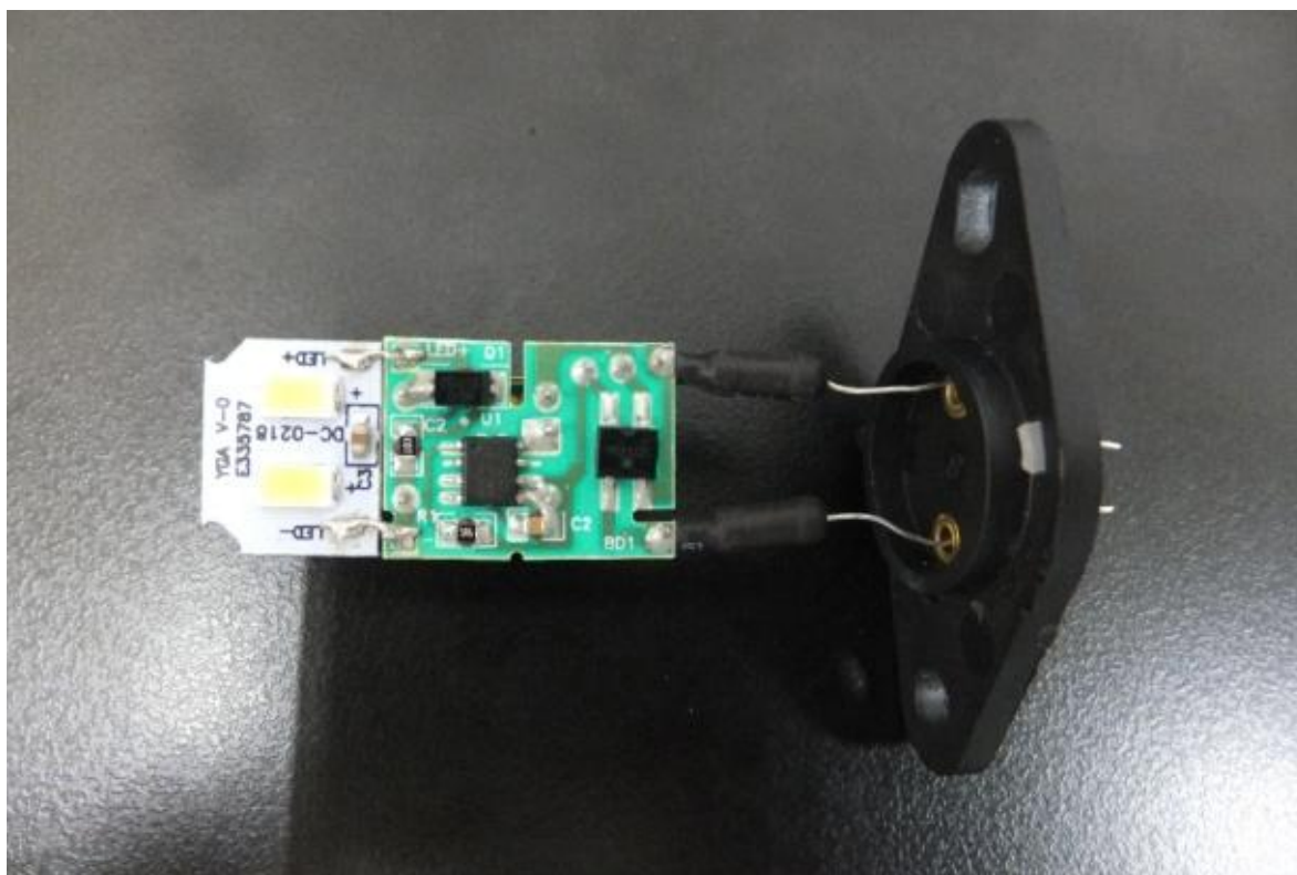
LED Lamp 2: PCB board- Bottom View
