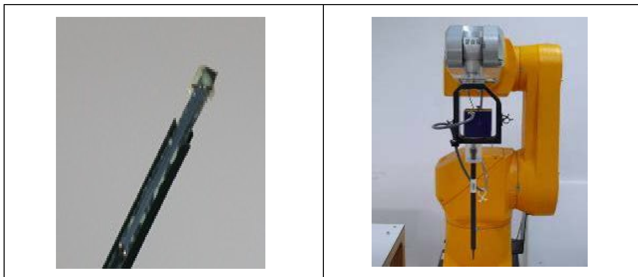
EX3DV4 E-field Probe
