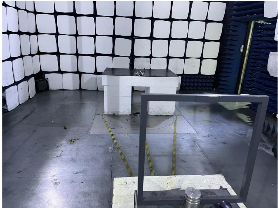
Radiation Emission Test Setup (Below 30MHz)
