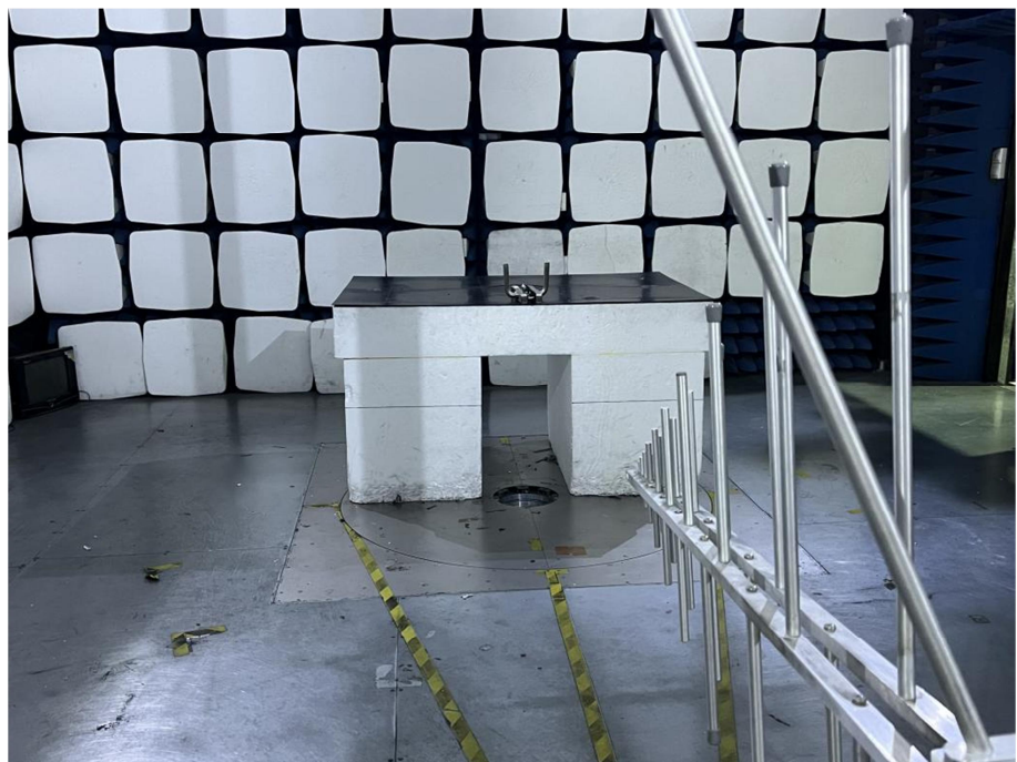
Radiation Emission Test Setup (30MHz to 1GHz)
