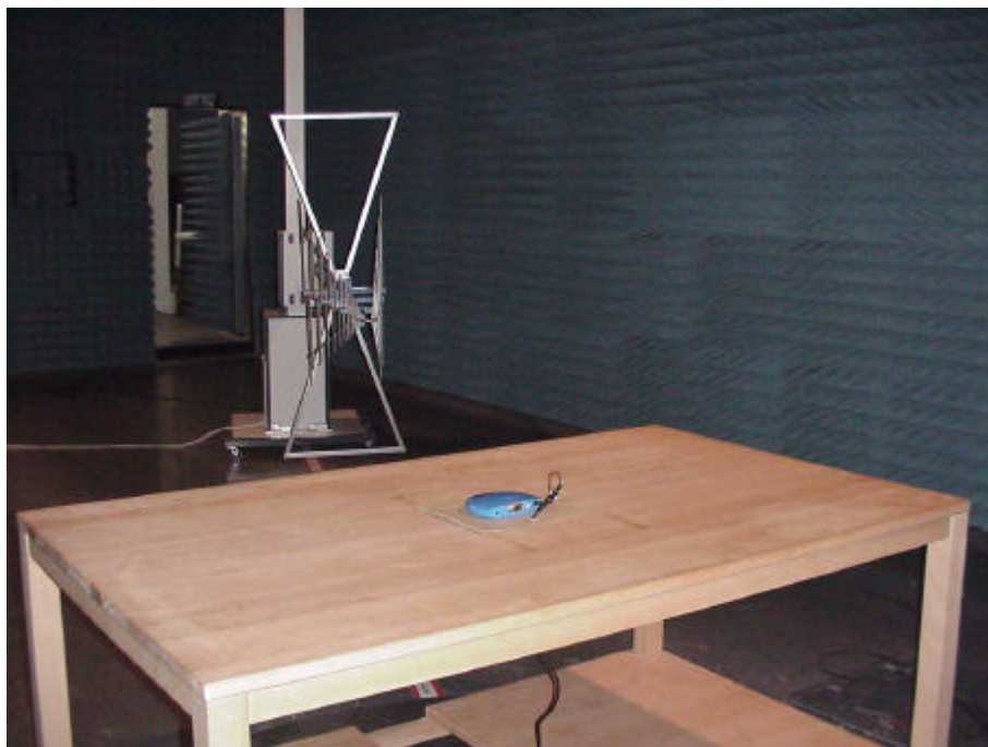
Picture 4 : Setup for radiated tests
