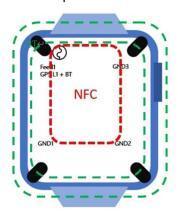
Antenna transmission frequency: 13.56MHz
