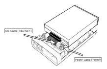
You should put the bottom case on the main frame of the FCD-524.You should fix the bottom case to the front cover of CD-ROM/DVD-ROM.
