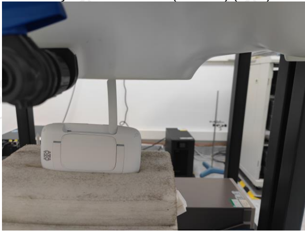
Body worn –Top-level(External)(0mm)
