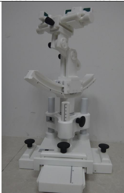
COMOSAR Mobile phone positioning system
