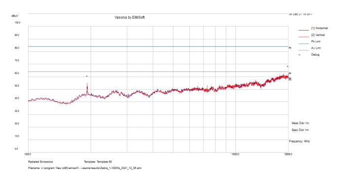
Correction Corrected Ant. Turntable Detector Ant. S.A. Reading Frequency Limit Margin Height Factor **Amplitude Polarity** Azimuth (Peak (MHz) (dBuV)  $(dB\mu V/m)$ (dB) (dB/m) $(dB\mu V/m)$ (degrees) (H/V) (cm) /Ave.) 17968.125 50.04 12.75 62.79 100 0 64 -1.21 Η Ave 1924.375 60.51 -5.54 54.97 V 0 -9.03 100 64 Ave
