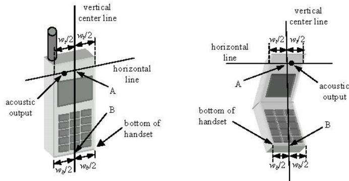
**Figure 8.3 Handset Vertical Center & Horizontal Line Reference Points**
