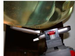
**Figure A.2 Right Head SAR Test Setup
