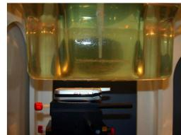
**Figure A.5 Body SAR Test Setup
