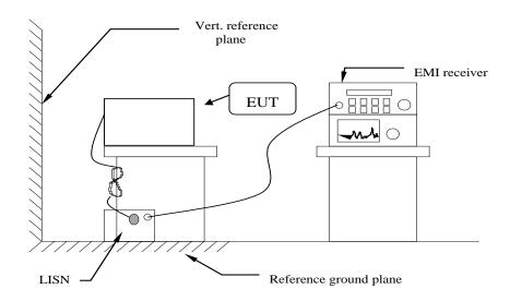
Note: the distance between LISN and Vertical reference plane is 40 cm and the distance between LISN and EUT is 80 cm.
