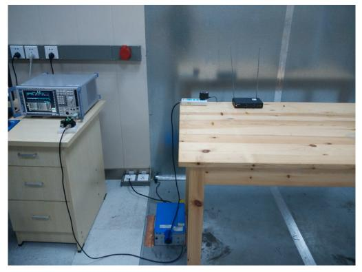
RADIATED EMISSION TEST SETUP
