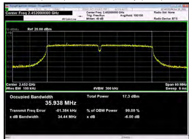
802.11n(HT40), Carrier frequency (MHz): 2452
