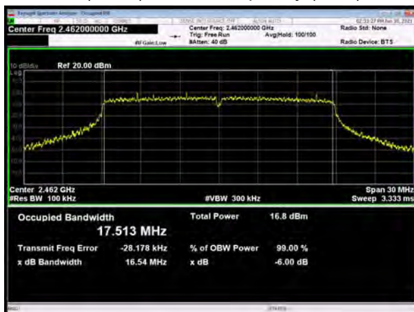
802.11n(HT20), Carrier frequency (MHz): 2462
