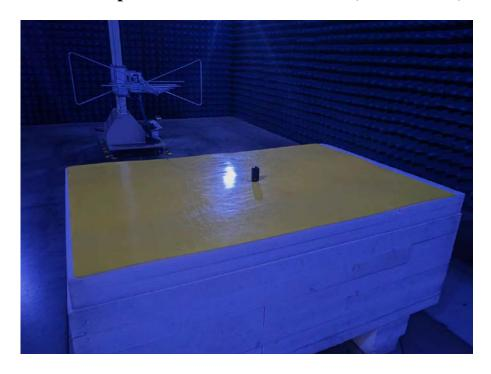
**Radiated Spurious Emissions Test View (Above 1GHz)**
