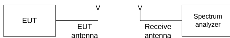
Figure 7.1.1 The 20 dB bandwidth test setup
