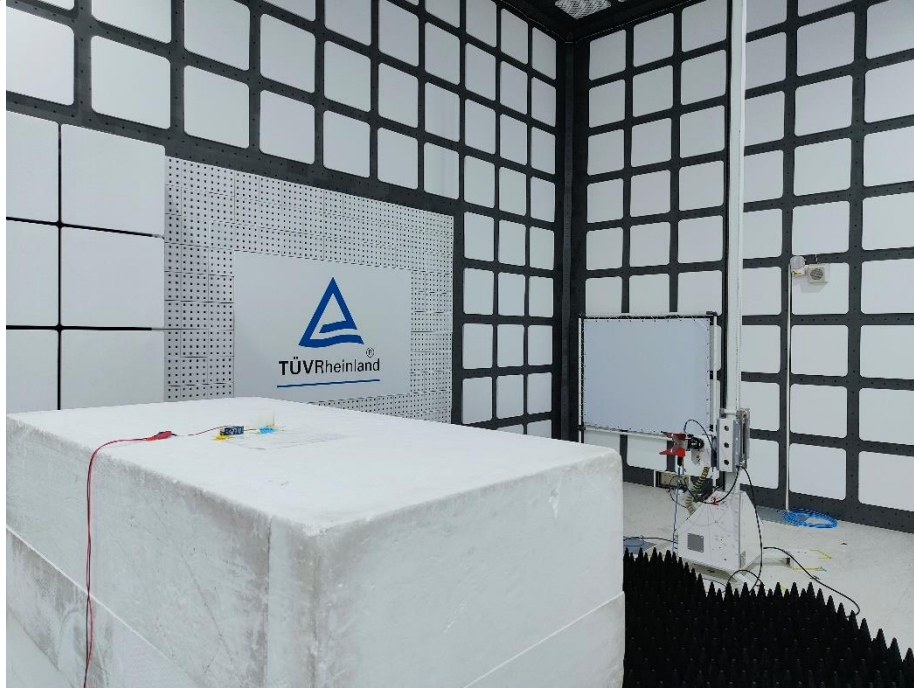
Photograph 6: Test Setup for Spurious Emissions (Back View 4)
