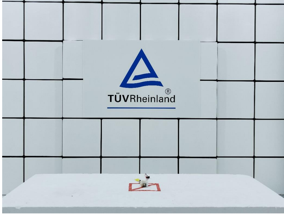
Photograph 2: Test Setup for Spurious Emissions (Front View 2)
