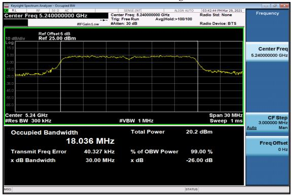
802.11n VHT40 26dB / 99% Band Width Test Data CH-Low
