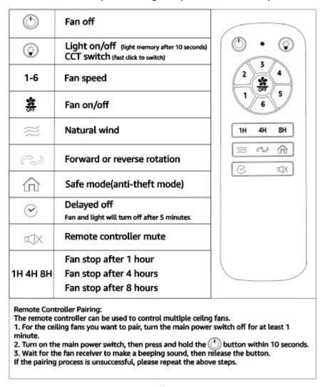
The wireless transmission frequency is: 433.92MHz
