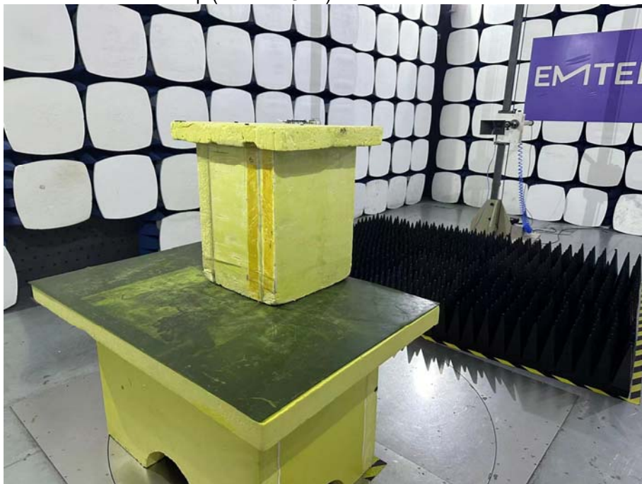
Spurious Emission Test Setup (Above 1GHz)
