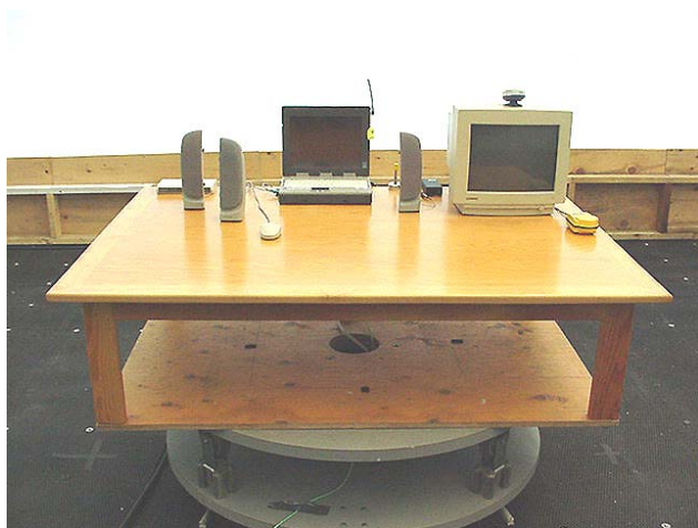
Photograph D.7-3 - Front of Radiated Emission Setup
