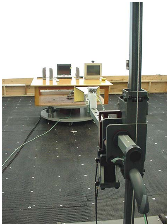
Photograph D.7-4 - Back of Radiated Emission Setup
