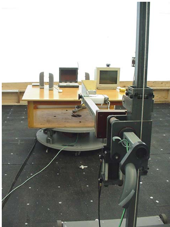
Photograph D.7-3 - Front of Radiated Emission Setup
