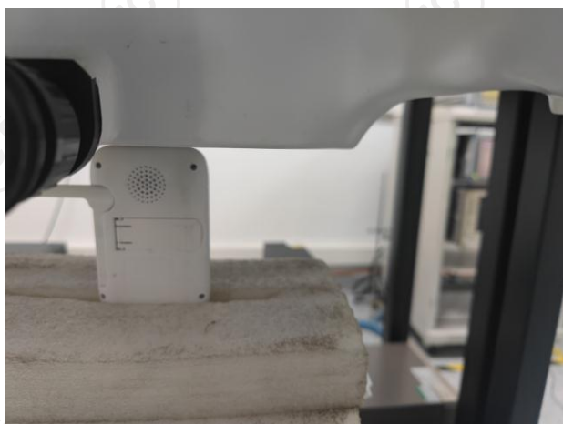
Body worn –Left-level(External) (0mm)
