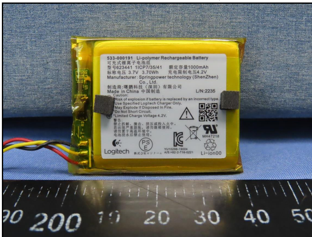
Battery (Brand: Springpower technology (ShenZhen) Co.,Ltd.; Model: 533-000191 or 623441)
