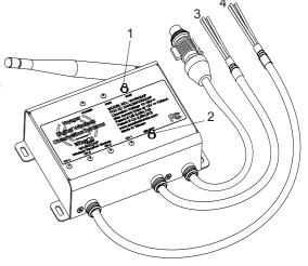
Make sure transmitter module is unpowered at first. Within 50 seconds of activating the pairing process on the receiver module, apply power to the transmitter module, and upon successful pairing, the receiver module and monitor screen will display "PAIRING SUCCESSFUL" message for 1~2 seconds with the status LED steady ON and display Camera image.
