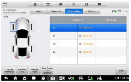
Figure 5-7 Sample Copy by OBD Function Main Screen
