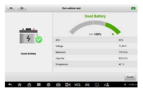
Figure 9-14 Sample Out-vehicle Test Result Screen
