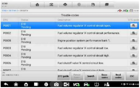
Figure 4-19 Sample DTC & FFD Screen
