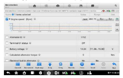
Figure 4-13 Sample Waveform Graph Mode Screen
