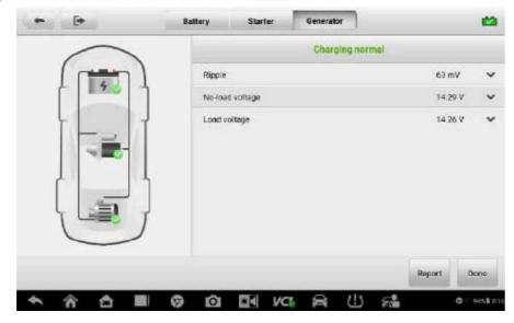
Figure 9-12 Sample Generator Test Result Screen
