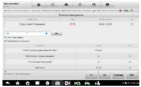
Figure 4-16 Sample Active Test Screen
