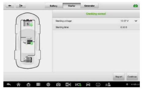
Figure 9-10 Sample Starter Test Result Screen
