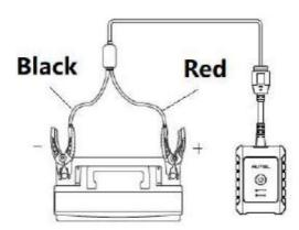
Figure 9-2 Connecting to a Battery
