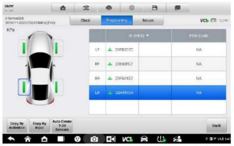
Figure 5-5 Sample Copy by Activation Function Main Screen
