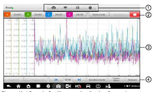
Figure 19-4 Sample Oscilloscope Application Screen Layout
