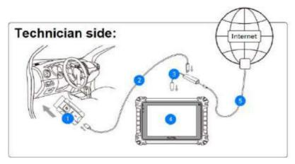
Figure 8-1 Sample connection diagram on Technician side
