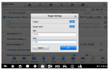
Figure 4-14 Sample Trigger Setting Dialog Box
