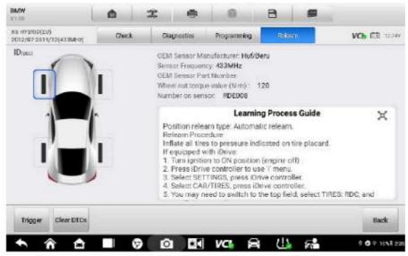
Figure 5-8 Sample Relearn Function Main Screen
