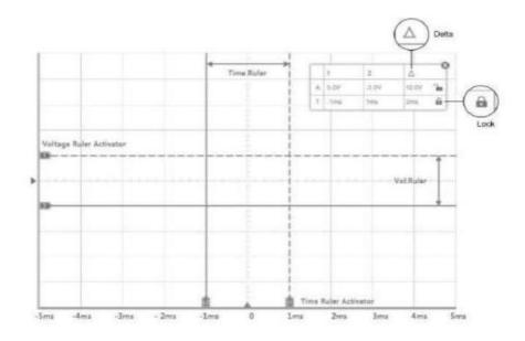
Figure 19-8 Measurement Rulers Display
