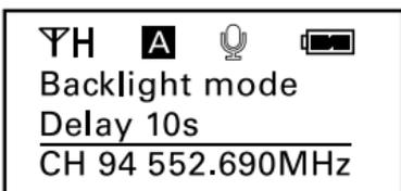
Set Backlight. Select ON, OFF or Delay 10 / 30 /60 seconds. Default is "Delay 10s."
