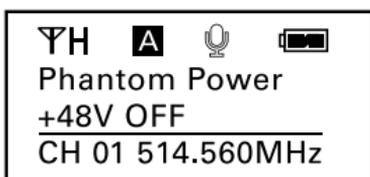
Set the microphone drive power supply (+48V). When set to ON, 48V phantom power is supplied to the connected microphone and the "+48V" indicator lights up. Default is "+48V OFF."
