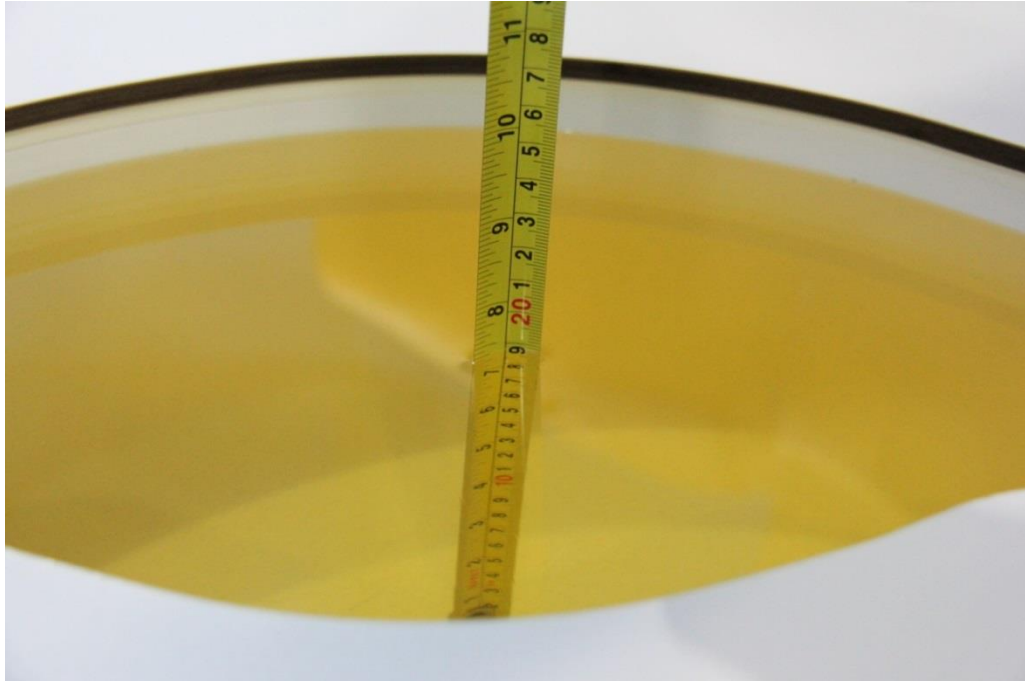
Picture 7-1: Liquid depth in the Flat Phantom(750MHz)
