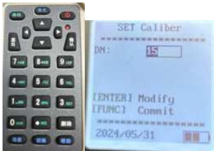
Figure 4: Setting the DN Size
