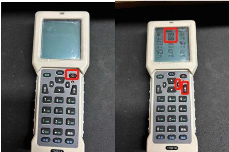
Figure 2: Power on the Handheld Device
