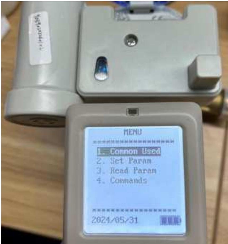
Figure 7: Configuring the MIU with the Handheld Device
