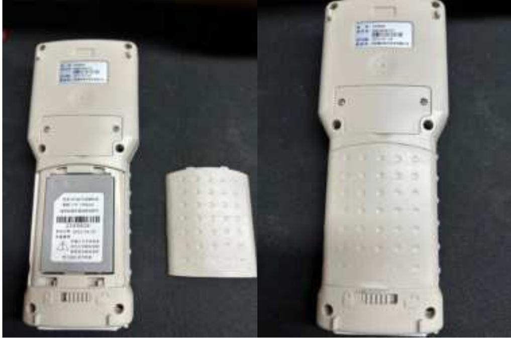
Figure 1: Install the battery to the Handheld Device
