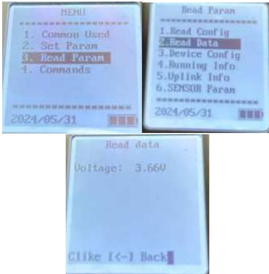
Figure 28: Reading of Battery Voltage
