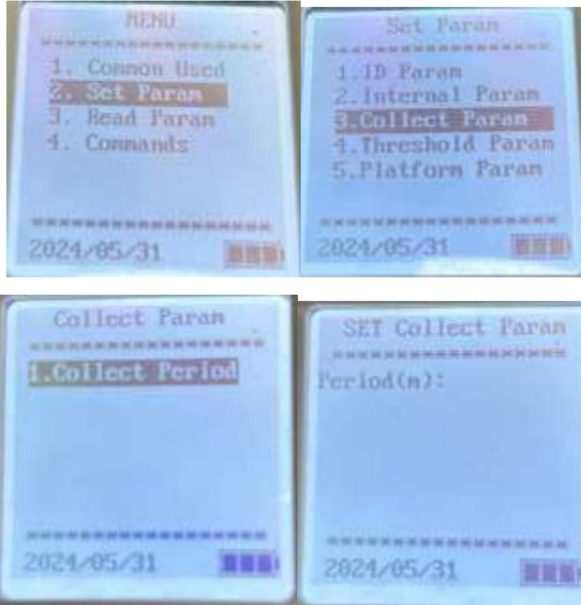
Figure 16: Setting the MIU data sampling interval
