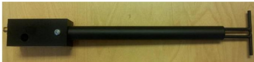
Figure 1 – MVG COMOSAR Validation Dipole
