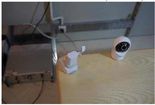
Radiated Emissions (30MHz-1GHz) Test Setup
