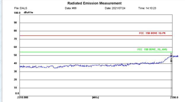
26(C) Site 966 Chamber Temperature: Polarization: Vertical
