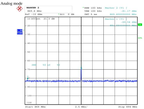
22.917 Marker 1 is from base station simulator Marker 2 is highest emission Channel 384
