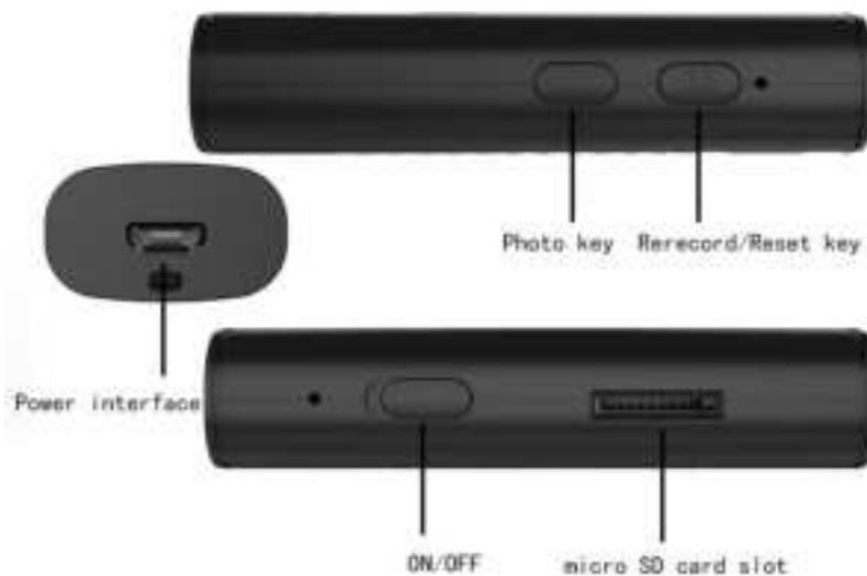
The blue indicator light is the recording indicator: recording -> blue light flashes slowly; stop recording —>Steady blue light;
