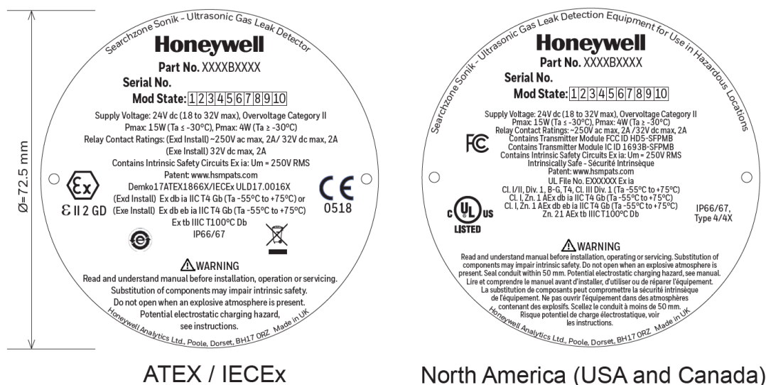
Figure 7: Example shows details of label of Search Platform Detectors. EU on the left, North America on the right.
