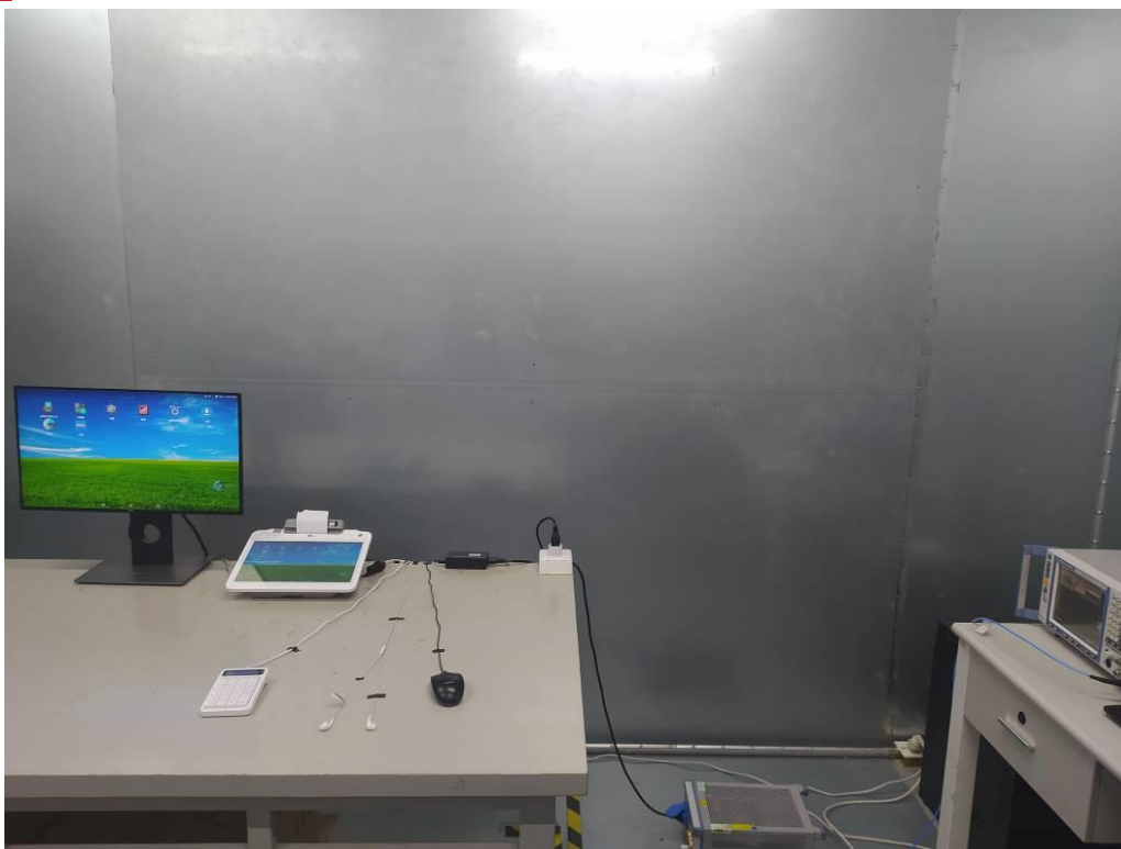
Fig. 3 Power line conducted emission setup photo
