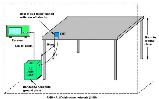
AE = Associated equipment EUT = Equipment under test
