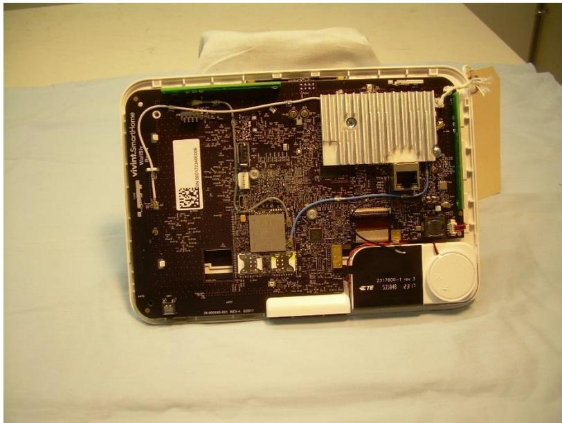
**Photograph 4 – View of the EUT with Rear Cover Removed Showing the Back Side of the Main PCB**
