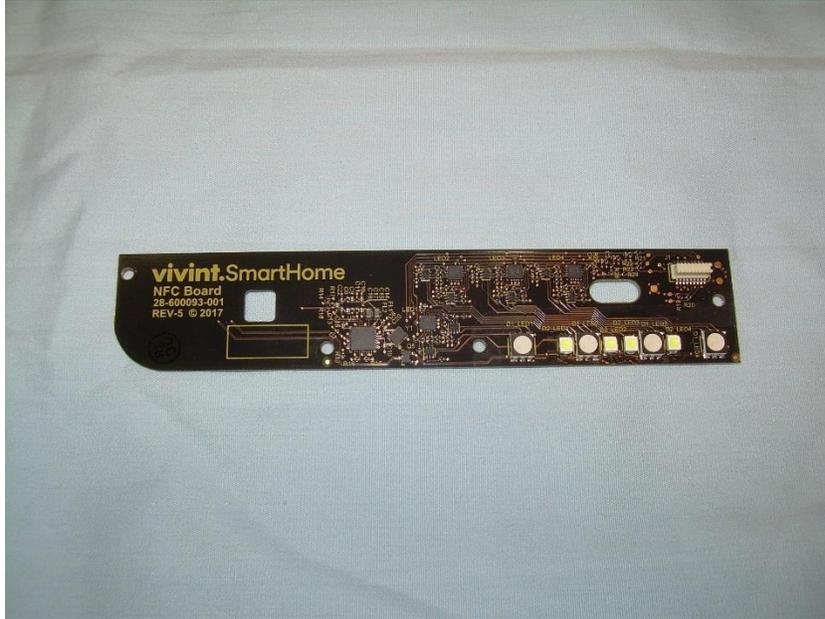
**Photograph 11 – View of the Component Side of the NFC PCB**
