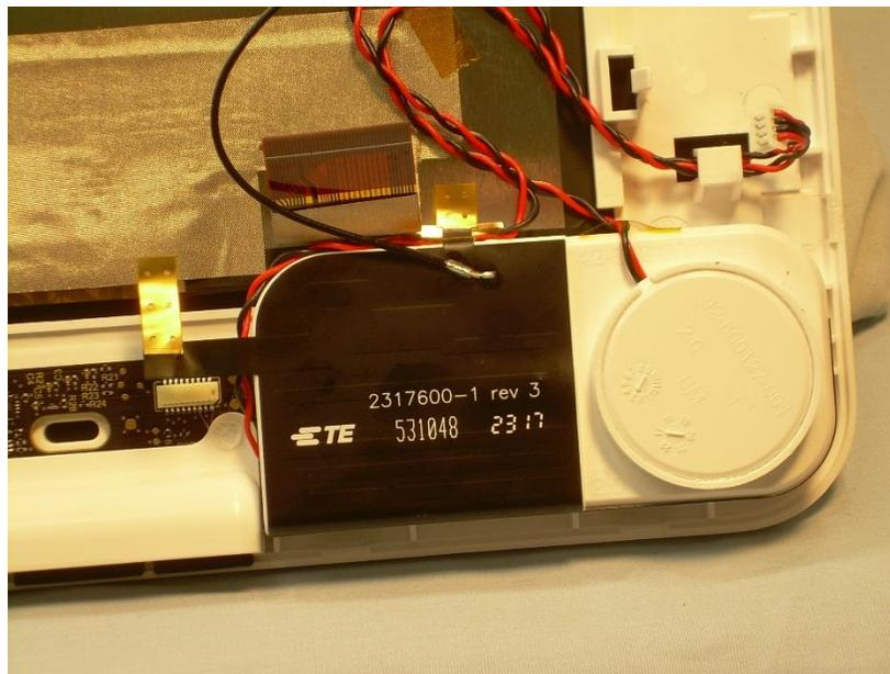
**Photograph 10 – View of the Speaker and 345 MHz Receiver Antenna**
