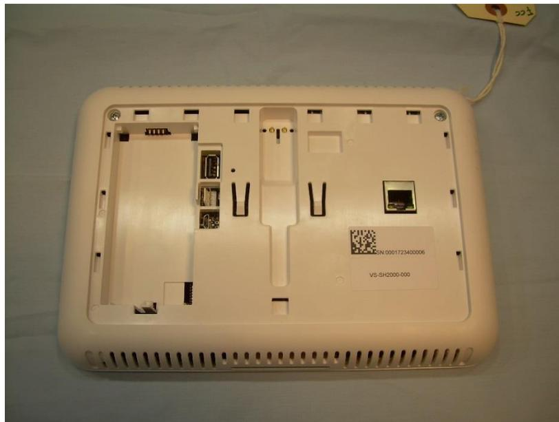
**Photograph 2 – View with the Battery and the Back Panel of the EUT Removed**
