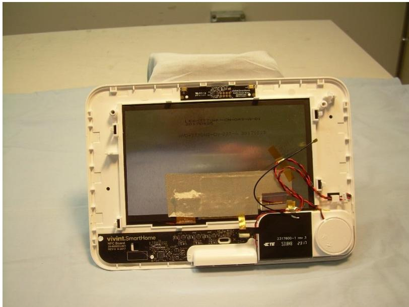
**Photograph 6 – View with the Main PCB Removed**
