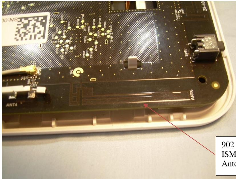
**Photograph 9 – View of the 902 -928 MHz Transceiver Antenna**
