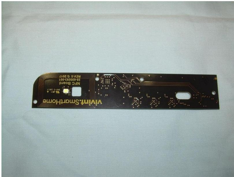
**Photograph 12 – View of the Trace Side of the NFC PCB**
