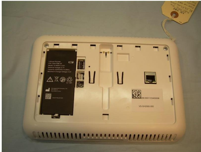
**Photograph 1 – View with the Back Panel of the EUT Removed**
