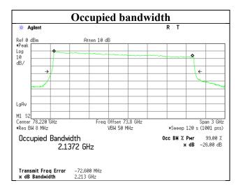
The measurement was performed with Peak detector and Max Hold since the duty cycle was not 100 %.
