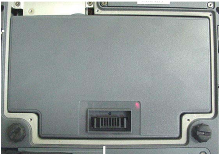
Internal Li-ion Battery 11.1 V, 3600 mAh (Model: T8M-E)
