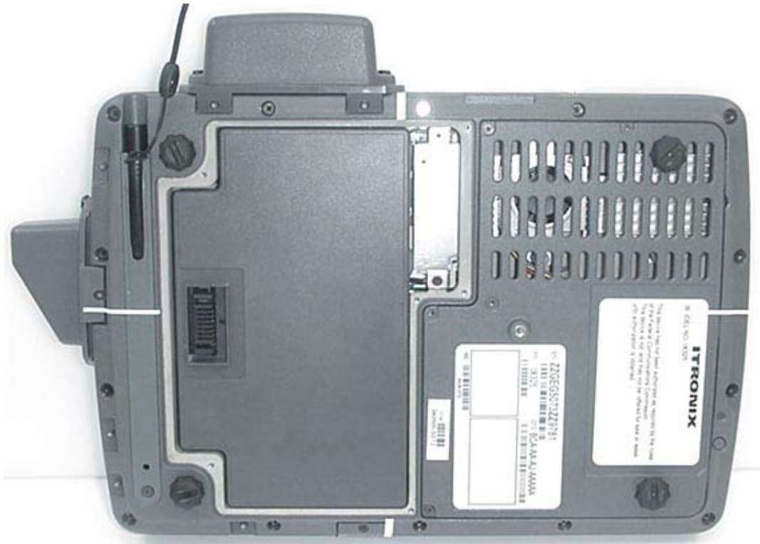
DUT with Internal Li-ion Battery 11.1 V, 3600 mAh (Model: T8M-E)
